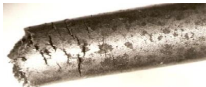
Crevice corrosion in stainless steel. Fasteners are at risk
